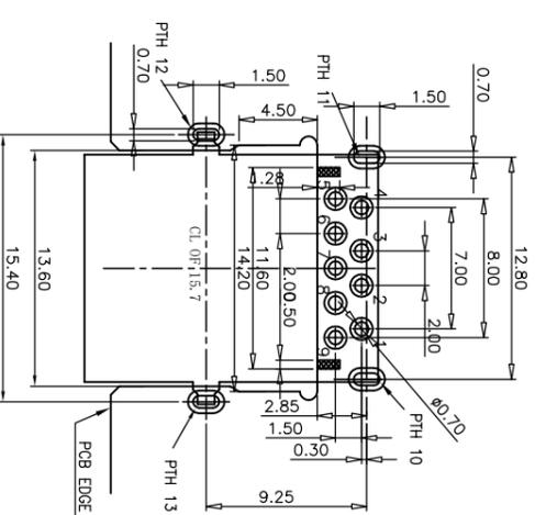
TOLERANCE: ±0.05, THICKNESS: 1.2mm
