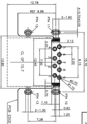
TOLERANCE:  $\pm 0.05$ , THICKNESS: 1.0~1.2mm
